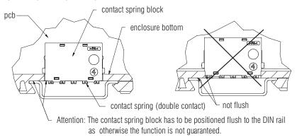
positioning of the contact spring block on the pcb; for enclosure series KS4400 and KS4460
