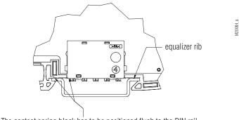
Attention: The contact spring block has to be positioned flush to the DIN rail as otherwise the function is not guaranteed.
